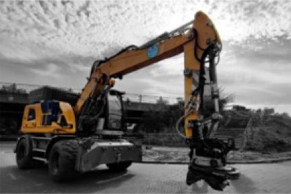
The two Liebherr 916 wheeled excavators belonging to contractor Jos Scholman are now powered by hydrogen fuel cells manufactured by Zepp Solutions based in Delft.
